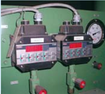
Pressure Switch EDS 1700 For wall-mounting.
